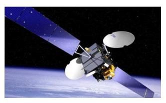
In the coming days, orbit raising manoeuvres will be performed to place the satellite in the Geostationary Orbit (36,000 km above the equator) by using the satellite's propulsion system in steps.
